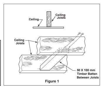
Always verify the ceiling structure is sound and capable of supporting a dead weight of at least 27 Kgs. The mounting bracket must be screwed directly to the rafters or a ceiling fan mounting device that has been correctly installed. All screws holding the bracket to the ceiling must penetrate half their length into the structural member. Concrete anchors must be suitable for longitudinal loads and installed according to the manufacturer's directions.
