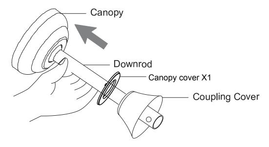
**Step 2** - Route all the wires from the motor through the down rod. Fit the down rod into the shaft coupler, align the pin holes and pass the motor support pin through the coupler and down rod. Secure the motor support pin with the R shaped cotter pin.
