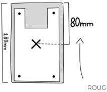
ROUGH IN LOCATION Hole size to fit cables, dimensions to be 30DIA mm.
